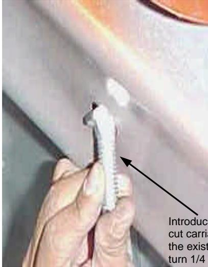
Introduce 1/2 x 1 1/2" cut carriage head bolt in the existing hole, then turn 1/4 to secure the head into the hole
