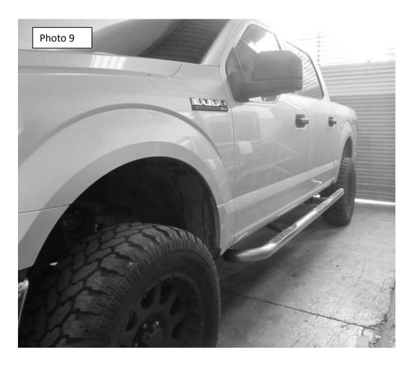
**8.** Repeat the above process to install the passenger side brackets and side bar.
