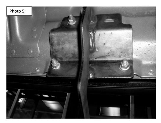
5. Attach the wheel to wheel to the front and rear bracket using (2) 1/2" x 2" hex bolts, (2) 1/2" flat washers and (2) 1/2" spring lock washers. Leave the nuts loose for final adjustment. (Photo 6 & 7)
