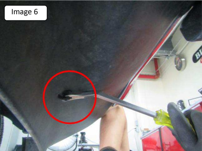
5. Locate and remove the factory bolt shown. Place auxiliary mounting bracket and secure usgin the bolt removed. Do not tighten. Image 7 y 8.
