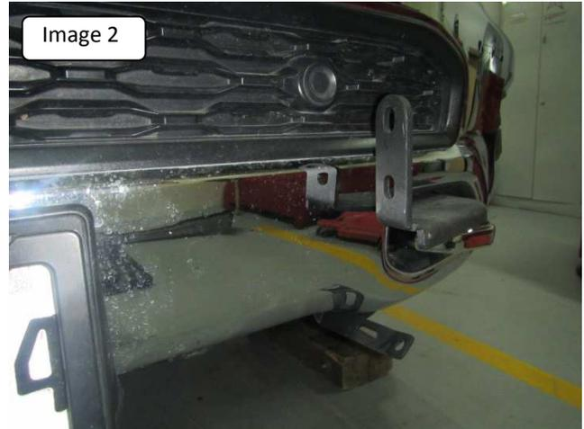
3. Place (2) 1/2" tab bolts from front of the main bracket to rear. Secure the main bracket to the bumper support using (2) 1/2 hex nuts, (2) 1/2" flat washers and (2) 1/2" lock washers. Image 3 & 4. **Note:** Leave the nuts loose for final adjustment.
