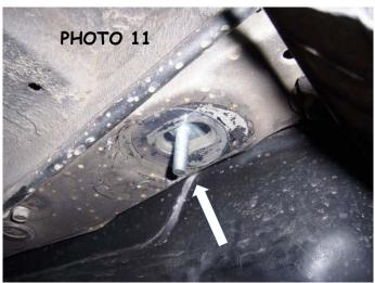
12.- Attach one of the rear brackets to the bottom of the frame using the 3/8" t-bolt, (1) 3/8" flat washer, (1)
