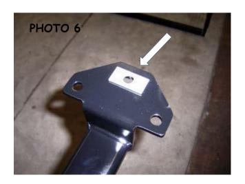
8.- Attach the opposite end of the front bracket to the auxiliary bracket using (1) 5/16" x 1" hex bolt, (1) 5/16"
