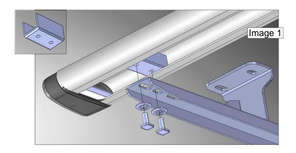
Align the side step with the vehicle an thigten the mounting brackets and the side step nuts and bolts. Remember to periodically check and retighten all nuts and bolts.
