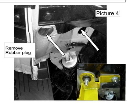
3. To install the rear mounting bracket, locate the abround hole and remove the rubber plug to expose the hole In the underside of the body at the rear of the vehicle. Picture 5
