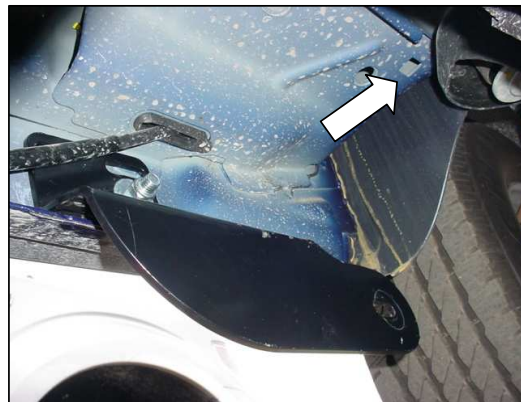
Insert into the square hole 5/16" bolt plate. Front driver's side shown.
