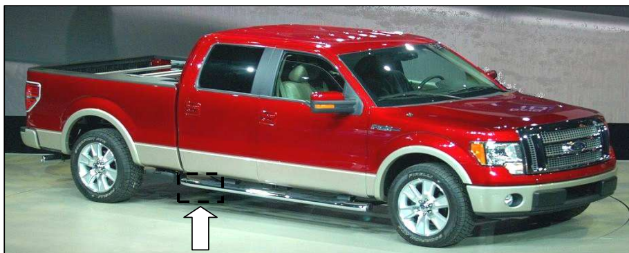
Section to install rear bracket.
