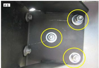
**Step-1** If use tow hook. Just loosen the nut from tow hook as shown. Leave loose the nut. ( Photo 7 )
