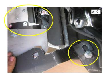
**Step-5** Align the holes and attach each factory bumper support bar to each of the replacement bumper support bracket using: (1)  $1/2 \times 1$  1/2" hex bolt, (1) 1/2" hex nut, (1) and (4) 1/2" flat washer. Leave the nuts and bolts loose for final adjustment. (Photo 11)
