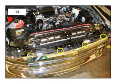
Step-3 Working from side to side gently pull outward to unsnap the clips and remove the grille, ( Photo 3 ).
