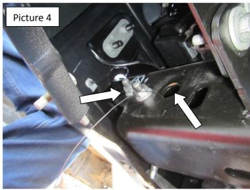
**4.** Attach the lower bracket to the side of the frame at bolt plate using 1/2" flat & lock washers and 1/2" hex nut, do not tighten. Attach to the existing bolts using the nuts removed. Picture 5. Repeat to install passenger side lower bracket. **NOTE:** The lower brackets must extend through the cut out opening made in the air dam.
