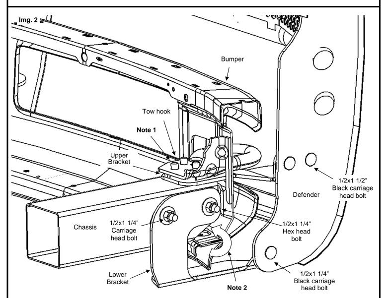
Note 1. To remove and install the tow hook's bolts you can use a wrench nut. Reach them from the lower side of the chassis.
