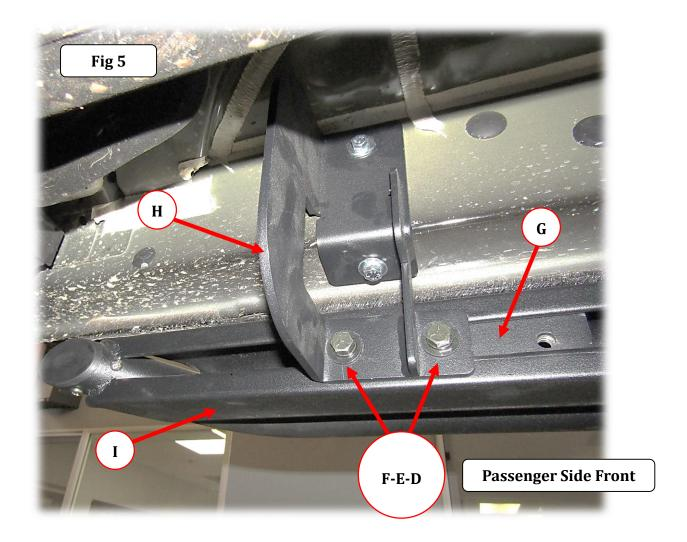
**Step-6**Tighten the bolts securing the mounting brackets to the body panel and the bolts securing the Dominator DSS side step to the mounting brackets.
