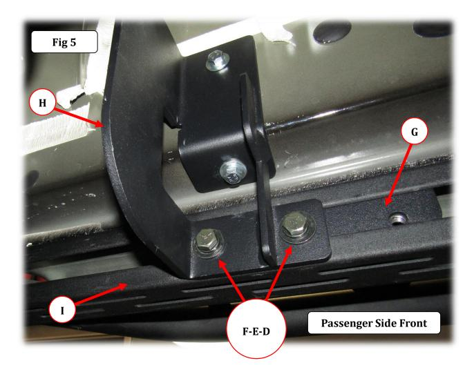
**Step-6** Tighten the bolts securing the mounting brackets to the body panel and the bolts securing the Dominator D6 side step to the mounting brackets.
