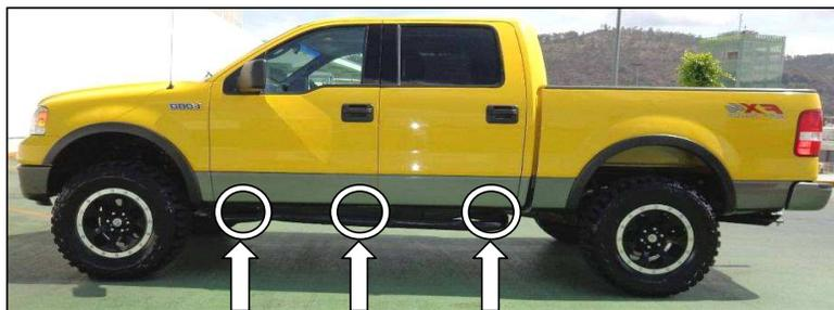
In this part, install each bracket on driver side.
