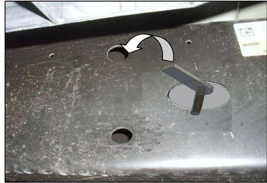
Insert the 3/8" threaded rod plate in the hole as shown. Place the middle auxiliary bracket A and attach with 3/8" bolts.
