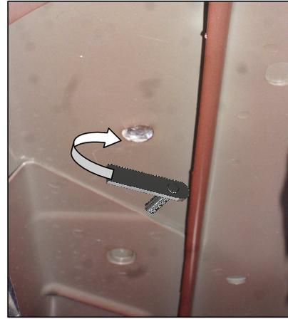
Insert the 3/8" threaded rod plate in the hole as shown.
