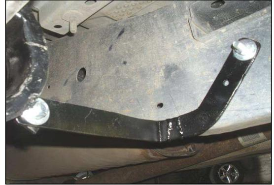
Shows the rear bracket assembly. Picture passenger side.
