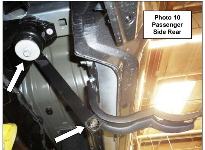
**Step-9** Attach the passenger side step to each of the brackets using (2) 5/16" x 1" hex bolts, (2) 5/16" lock washers and (2) 3/8" flat washers, (**Illustration 1**).
