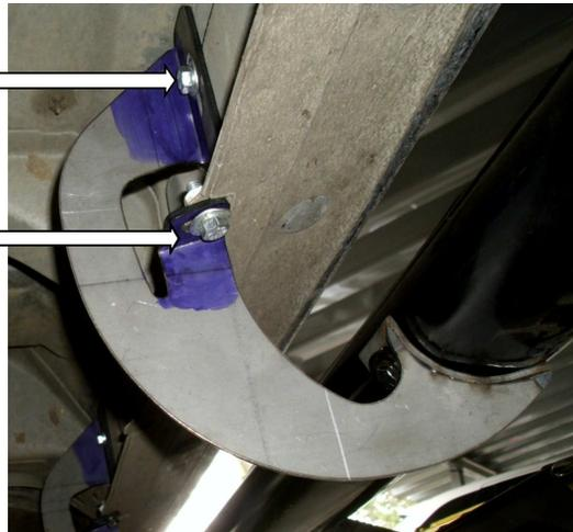
7. Oval side bar 4", place on brackets and attach with: 5/16" hex head bolt, 3/8" Flat washer, and Flat lock 5/16" **PHOTO 6** Repeat for the opposite side. Leave loose.
