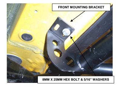
**STEP 4.** Repeat the above steps to install the driver side sidestep.
