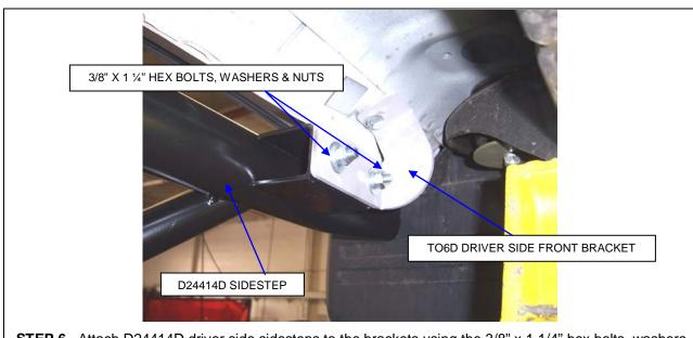
**STEP 6.** Attach D24414D driver side sidesteps to the brackets using the 3/8" x 1 1/4" hex bolts, washers and nuts.
