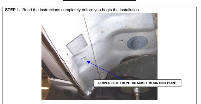
**STEP 2.** This installation uses (3) brackets per side. Begin by installing the driver side front bracket. Locate the threaded hole in the underside body panel.
