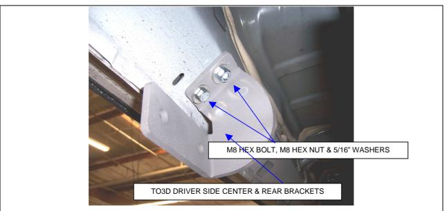
**STEP 5.** Loosely attach the TO3D center and rear brackets, to the body panel using the M8 hex bolts, M8 hex nuts and 5/16" washers.
