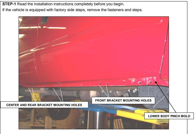
**STEP-2** This installation uses three mounting brackets per side. Beginning with the passenger side, locate the holes in the rocker panel and lower body pinch mold.
