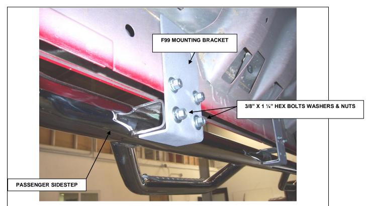
**STEP-4** Position the passenger sidestep up to the mounting brackets and loosely attach it to the brackets using the 3/8" x 1 1/4" hex bolts, washers and nuts as shown.
