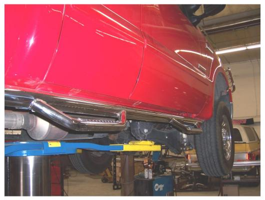
**STEP-5** Align sidestep with the body, and then tighten all mounting bracket and sidestep nuts and bolts. Repeat the above steps to install the driver side mounting brackets and sidestep.
