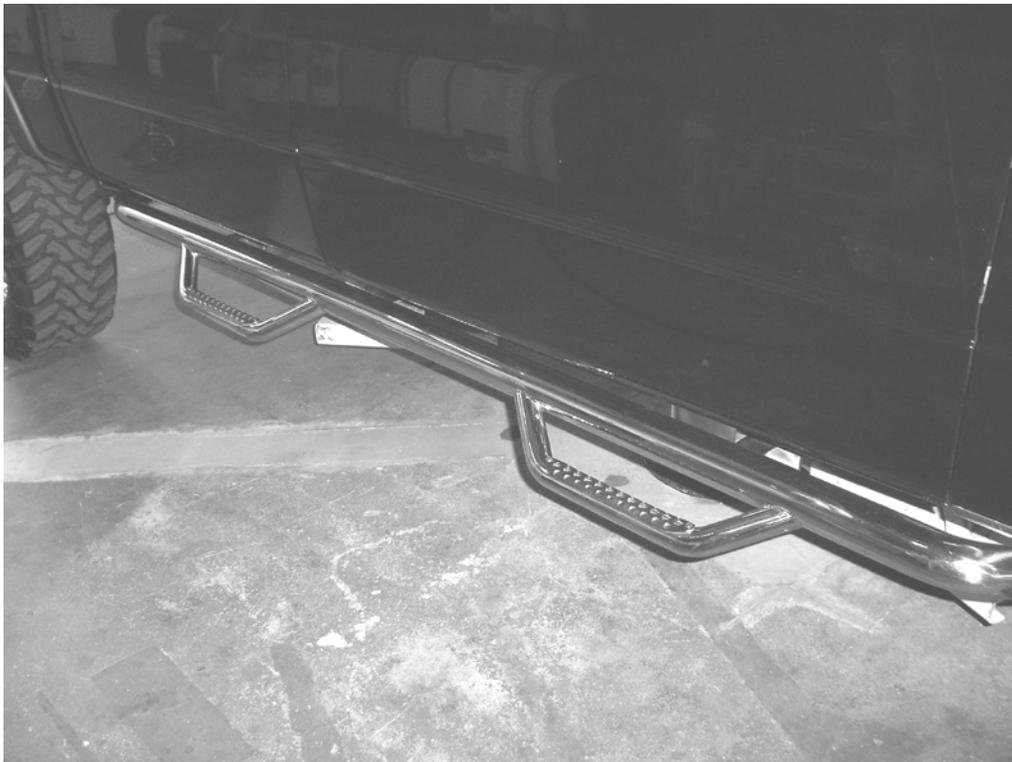
**STEP 5.** Align sidestep with the body, and then tighten all mounting bracket and sidestep nuts and bolts.
