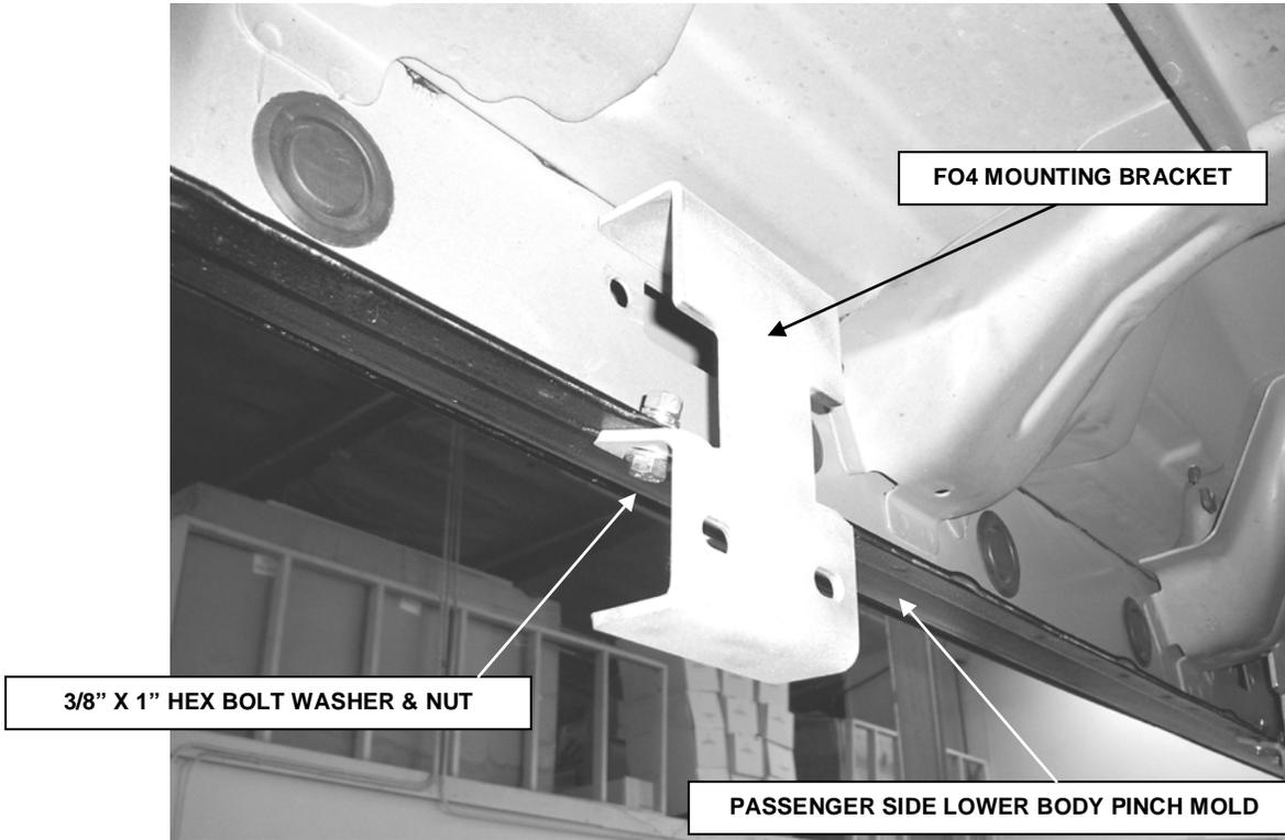
**STEP 3.** Loosely attach the flange of the mounting brackets to the bottom of the lower body pinch mold using the 3/8" x 1" hex bolts, washers, and nuts as shown.
