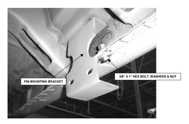
**STEP 6.** Loosely attach the flange of the mounting bracket to the bottom of the lower body pinch mold using the 3/8" x 1" hex bolts, washers, and nuts.
