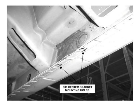
**STEP 5.** Locate the holes in the lower body pinch mold for the center-mounting bracket.
