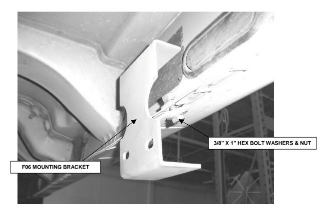
**STEP 8.** Loosely attach the flange of the mounting bracket to the bottom of the lower body pinch mold using the 3/8" x 1" hex bolts, washers, and nuts.
