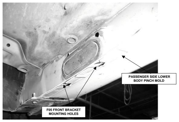
**STEP 3.** Beginning with the passenger side, locate the holes in the lower body pinch mold for the front mounting bracket.
