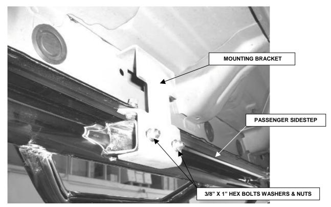
**STEP 9.** Position the passenger sidestep up to the mounting brackets and loosely attach it to the brackets using the 3/8" x 1" hex bolts, washers and nuts as shown.
