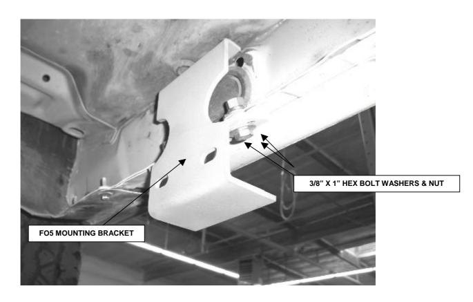
**STEP 4.** Loosely attach the flange of the front mounting bracket to the bottom of the lower body pinch mold using the 3/8" x 1" hex bolts, washers, and nuts as shown.
