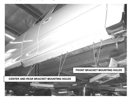
**STEP 2.** This installation uses three mounting brackets per side.
