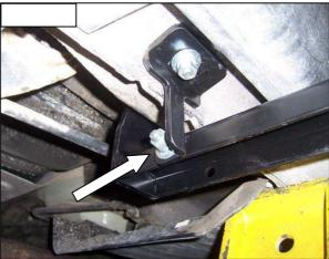
11. Adjust the driver side, side bar on top of the brackets and align and align the side bar with the vehicle. Position the clamp brackets inside the opening of the side bar and align the clamp bracket threads with the slot in the bracket. Attach the side bar to each of the brackets using the clamp brackets, using (2) 5/16" square head bolt, (2) 5/16" flat washer, (2) 5/16 lock washer. Leave loose. **Photo 15.**
