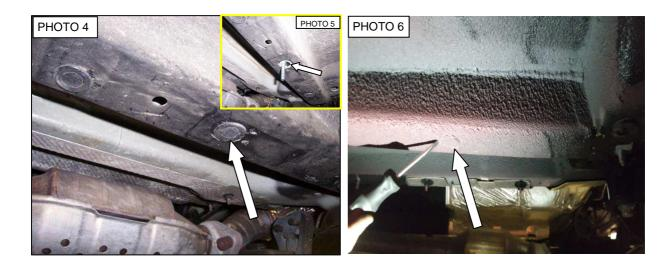
**4.** Attach the passenger side front bracket to the bottom of the frame using 3/8" T bolt (1) 3/8" flat washer (1) 3/8" lock washer and (1) 3/8" hex nut. **Photo 7.** Leave loose.
