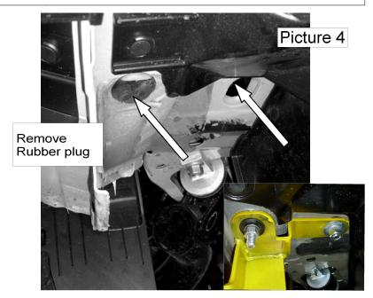
3. To install the rear mounting bracket, locate the abround hole and remove the rubber plug to expose the hole In the underside of the body at the rear of the vehicle. Picture 5
