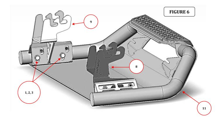
**Step-8** With assistance align and hold the RC3 front guard in the desired position on the vehicle, then tighten all OEM and supplied nuts and bolts.
