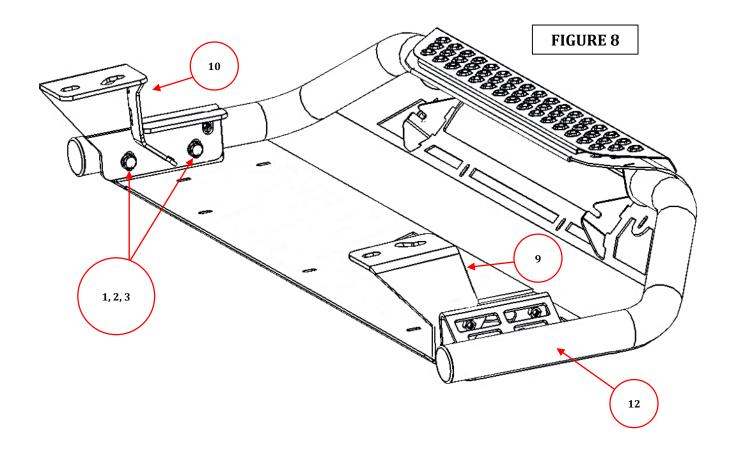
**Step-10** With assistance align and hold the RC3 front guard in the desired position on the vehicle, then tighten all OEM and supplied nuts and bolts.
