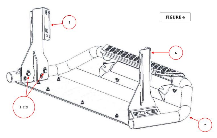
**Step-6** With assistance align and hold the RC3 front guard in the desired position on the vehicle, then tighten all OEM and supplied nuts and bolts.
