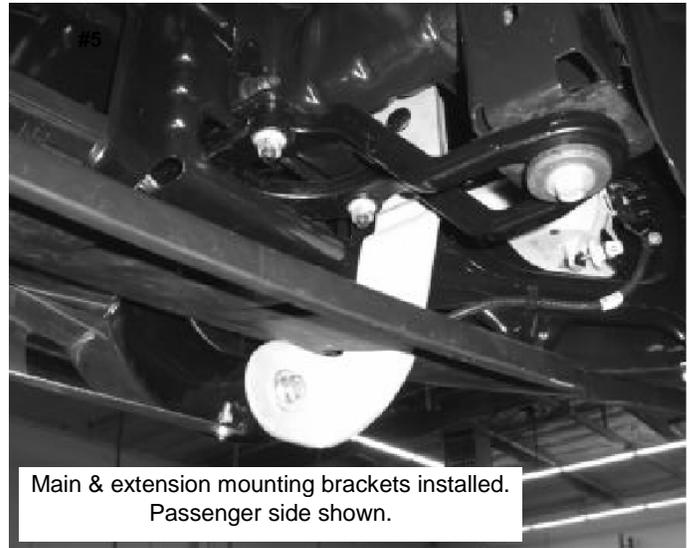
4. Position the passenger side main mounting bracket over the studs and secure the bracket to the frame using the (2) factory nuts. Do not tighten. Picture 3.
