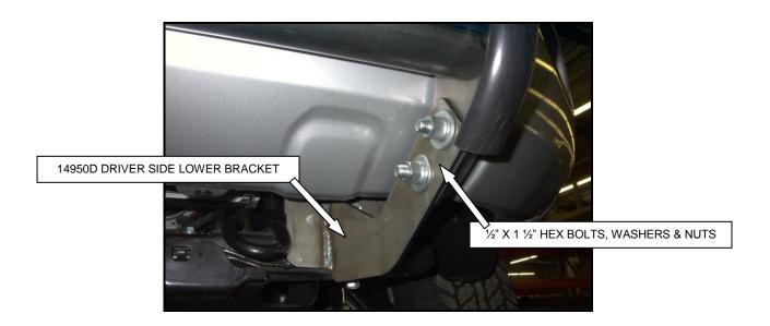
**STEP -7** ATTACH THE GRILLE GUARD ASSEMBLY TO THE OUTSIDE OF THE LOWER MOUNTING BRACKETS USING THE 1/2° X 1 1/2° HEX BOLTS, WASHERS, AND NUTS.
