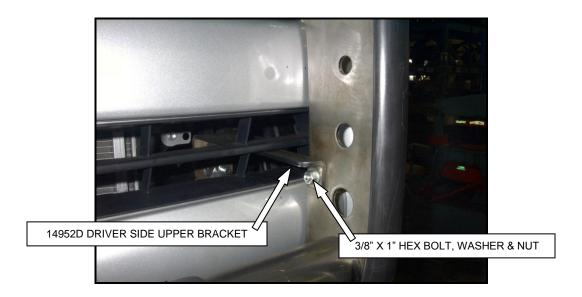
**STEP -8** ATTACH THE GRILLE GUARD ASSEMBLY TO THE UPPER MOUNTING BRACKETS USING THE 3/8" X 1" B HEX BOLTS, WASHERS, AND NUTS. ALIGN THE GRILLE GUARD ASSEMBLY WITH THE FRONT OF THE VEHICLE AND TIGHTEN ALL MOUNTING NUTS AND BOLTS.
