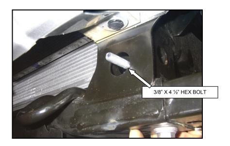
STEP -2 SLIDE THE  $\frac{1}{4}$ " THICK WASHER OVER  $\frac{3}{8}$ " X  $\frac{4}{2}$ " HEX BOLT. INSERT THE BOLT THROUGH THE HOLES IN THE BOXED FRAME SECTION WITH THE THREADS EXTENDING OUTWARD AS SHOWN.
