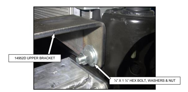
**STEP- 6** LOOSELY ATTACH 14952D UPPER MOUNTING BRACKET TO THE FRAME USING THE 1/2" X 1 1/2" HEX BOLT, WASHERS, AND NUT. REPEAT THE INSTALLATION FOR THE PASSENGER SIDE UPPER MOUNTING BRACKET.
