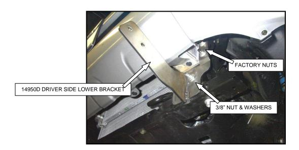
**STEP -3** POSITION 14950D LOWER MOUNTING BRACKET OVER THE STUDS, AND 3/8" HEX BOLT. LOOSELY ATTACH THE BRACKET TO THE FRAME USING THE FACTORY NUTS, 3/8" HEX NUT AND WASHER AS SHOWN. REPEAT THE ABOVE FOR THE PASSENGER SIDE LOWER MOUNTING BRACKET.
