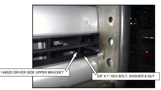
**STEP- 8** ATTACH THE GRILLE GUARD ASSEMBLY TO THE UPPER MOUNTING BRACKETS USING THE 3/8" X 1" B HEX BOLTS, WASHERS, AND NUTS. ALIGN THE GRILLE GUARD ASSEMBLY WITH THE FRONT OF THE VEHICLE AND TIGHTEN ALL MOUNTING NUTS AND BOLTS.
