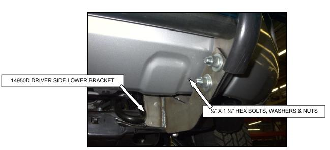
**STEP-7** ATTACH THE GRILLE GUARD ASSEMBLY TO THE OUTSIDE OF THE LOWER MOUNTING BRACKETS USING THE 1/2" X 1 1/2" HEX BOLTS, WASHERS, AND NUTS.
