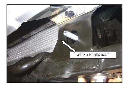
**STEP -2** SLIDE THE 1/4" THICK WASHER OVER 3/8" X 41/2" HEX BOLT. INSERT THE BOLT THROUGH THE HOLES IN THE BOXED FRAME SECTION WITH THE THREADS EXTENDING OUTWARD AS SHOWN.
