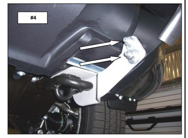
STEP-6 ALIGN THE GRILLE GUARD ASSEMBLY WITH THE FRONT OF THE VEHICLE AND TIGHTEN ALL NUTS AND BOLTS.
