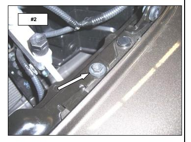
**STEP-4** ATTACH THE DRIVER SIDE UPPER BRACKET TO THE BUMPER USING (1) 6M X 20M HEX BOLT, (1) 6M LOCK WASHER AND (1) 6M FLAT WASHER. LEAVE THE BOLT LOOSE FOR FINAL ADJUSTMENT. **PHOTO #3**
