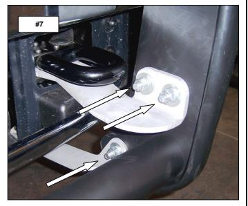
**STEP-9** ALIGN THE GRILLE GUARD ASSEMBLY WITH THE FRONT OF THE VEHICLE AND TIGHTEN ALL NUTS AND BOLTS.
