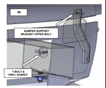
**STEP 7.** ATTACH THE AUXILIARY UPPER BRACKET TO THE BUMPER SUPPORT USING M8 X 40M HEX BOLT AND 5/16" FLAT WASHER, AND TO THE FRAME USING THE 3/8" T-BOLT, FLAT WASHER, LOCK WASHER AND HEX NUT. DO NOT TIGHTEN. **SEE DIAGRAM #7**
