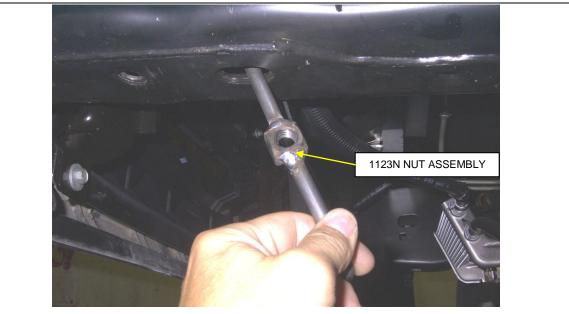
**2 WHEEL DRIVE MODELS**) TO ATTACH THE LOWER MOUNTING BRACKET, POSITION ONE OF THE 1123N NUT ASSEMBLIES UP THROUGH THE LARGER HOLE IN THE BOTTOM OF THE FRAME. ALIGN THE NUTS WITH THE TWO MATCHING HOLES IN THE FRAME, AND ATTACH THE MOUNTING BRACKET USING THE <sup>1</sup>/<sub>2</sub>" X 1 <sup>1</sup>/<sub>2</sub>" BOLTS, AND WASHERS SUPPLIED.
