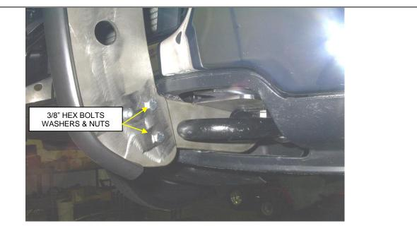
**STEP 4.** ATTACH THE GRILLE GUARD ASSEMBLY TO THE LOWER MOUNTING BRACKETS USING THE 3/8" X 1 1/4" HEX BOLTS, WASHERS AND NUTS. DO NOT TIGHTEN.
