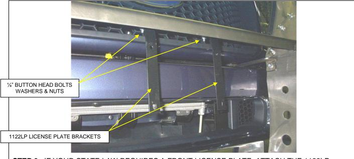
**STEP 6.** IF YOUR STATE LAW REQUIRES A FRONT LICENSE PLATE, ATTACH THE 1122LP BRACKETS, AND LICENSE PLATE TO THE GRILLE GUARD CENTER PLATE USING THE ¼" BUTTON HEAD BOLTS, WASHERS, AND NUTS.
