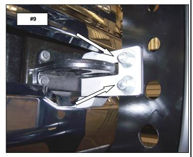
**STEP-8** ATTACH THE CENTER PLATE BRACKETS TO THE UPPER BRACKETS USING (2) 3/8" X 1" HEX BOLTS, (2) FLAT WASHERS, (2) LOCK WASHERS AND (2) HEX NUTS. **PHOTO #10**
