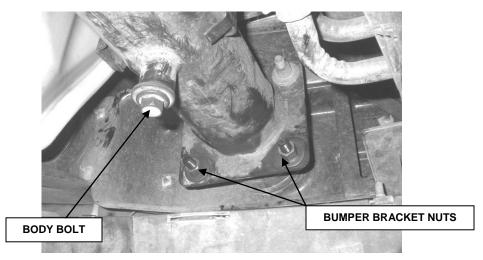
**STEP 1.** BEGINNING WITH THE DRIVER SIDE, LOCATE AND REMOVE THE BODY MOUNTING BOLT FROM THE BOTTOM OF THE FRAME, AND THE HEX NUTS THAT SECURE THE BUMPER BRACKET TO THE FRAME.
