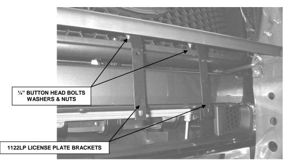
**STEP 12.** IF YOUR STATE LAW REQUIRES A FRONT LICENSE PLATE, ATTACH THE 1122LP BRACKETS, AND LICENSE PLATE TO THE GRILLE GUARD CENTER PLATE USING THE  $\frac{1}{2}$ " BUTTON HEAD BOLTS, AND NUTS.
