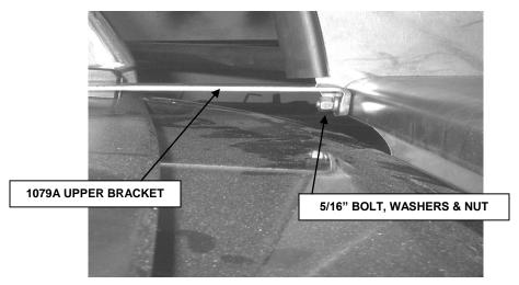
**STEP 9.** ATTACH THE CENTER PLATE OF THE GRILLE GUARD ASSEMBLY TO THE UPPER MOUNTING BRACKETS USING THE 5/16" X 1" HEX BOLTS, WASHERS, AND NUTS.
