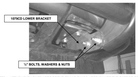
**STEP 8.** ATTACH THE LOWER LEGS OF THE GRILLE GUARD ASSEMBLY TO THE OUTSIDE OF THE LOWER MOUNTING BRACKETS USING THE 1/2" X 1 1/2" HEX BOLTS, WASHERS, AND NUTS.
