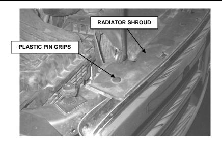
STEP 4. OPEN THE HOOD AND REMOVE THE PLASTIC PIN GRIPS AND PLASTIC RADIATOR SHROUD.
