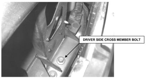
$\mbox{\bf STEP 6.}$  REMOVE THE CROSS MEMBER BOLT. ACCESS THE BOLT BY PULLING OUTWARD ON THE TOP OF THE GRILLE.
