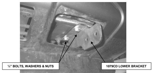
STEP 3. ATTACH 1079CD LOWER BRACKET TO THE BOTTOM OF 1079BD USING THE  $\frac{1}{2}$ " X 1  $\frac{1}{2}$ " BOLTS WASHERS AND NUTS AS SHOWN. REPEAT THE ABOVE STEPS FOR THE PASSENGER SIDE LOWER MOUNTING BRACKET.
