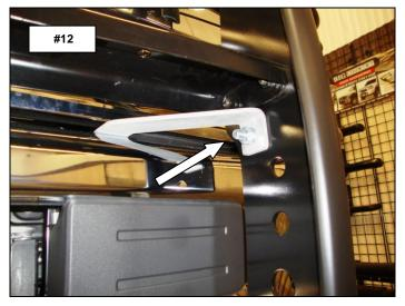
**Step-10** If your state law requires a front license plate, attach the supplied bracket to the upper set of holes in the vehicle bracket using the factory license plate attachment screws. Attach the license plate to the supplied bracket using (2)  $\frac{1}{4}$ " x  $\frac{3}{4}$ " hex bolts and (2)  $\frac{1}{4}$ " hex nuts, **(Photo 13)**.
