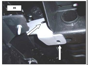
**Step-4** position the tow hook inside the frame, align the bracket and tow hook with the holes in the frame and reinstall the tow hook bolts and nut. Leave the tow hook bolts and nut loose for final adjustment. **Photo #5 & #6**
