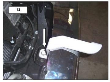
**Step-9** Attach the grille and brush guard assembly to the out side of the brackets using the ½" x 1 ¼" carriage bolts, ½" flat washers, ½" lock washers and ½" hex nuts for the lower brackets and the 3/8" x 1 ¼" hex bolts, 3/8" flat washers, 3/8" lock washers and 3/8" hex nuts for the upper brackets. Align the grille and brush guard assembly with the vehicle and tighten all nuts and bolts **Photo #13 & Photo #14**
