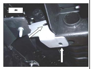
**Step-4** position the tow hook inside the frame, align the bracket and tow hook with the holes in the frame and reinstall the tow hook bolts and nut. Leave the tow hook bolts and nut loose for final adjustment.
