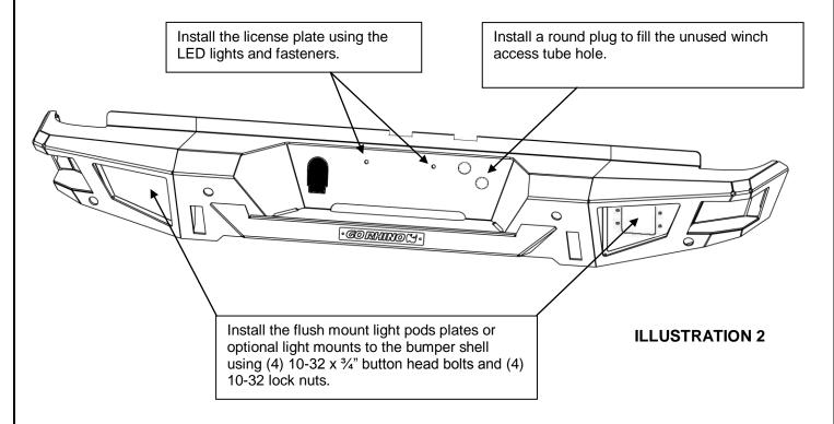
Step-16 Remember to check and retighten all factory and supplied nuts and bolts periodically.
