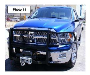
Step-9 Align the winch guard with the vehicle and tighten the factory and supplied nuts and bolts,
