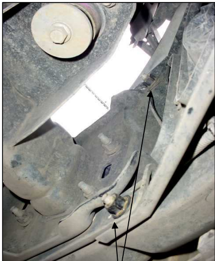
Nuts to remove for the installation of main bracket, passenger side.
