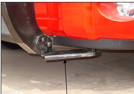
Main bracket installed, driver side.
