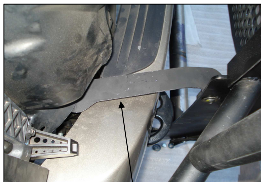
Auxiliary bracket installed, passenger side.
