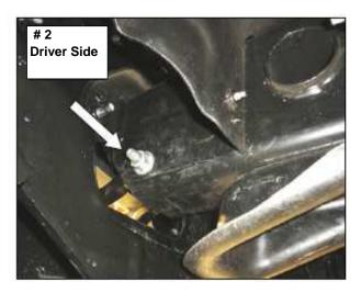
**Step-2** from the tow hook opening, slide the vehicle attachment end of the driver side upper bracket under the frame, rotate the bracket and position upper attachment hole in the bracket over the shank of the front tow hook bolt and reinstall the nut, ( **Photo 3 & 4** ).
