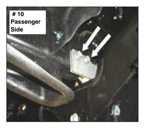
**Step - 6** Identify the holes to use for your vehicle (**Photo 11**) With assistance, position and attach the Grille Guard to the outside of each upper bracket using (2) 1/2 x 1 1/2" hex bolt, (2) 1/2" Flat washers, (2) 1/2" lock washers, (2) 1/2" hex nuts. Leave the nuts and bolts loose for final adjustment.
