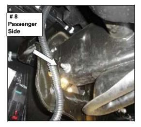
**Step -5** From the tow hook opening, side the vehicle attchment end of the passenger side upper bracket under the frame,rotate the bracket and aling the holes in the bracket with the holes in the side of the frame and reinstall the tow hook front bolt and nut, then the rear bolt, (**Foto 9 & 10**).
