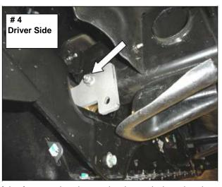
**Step- 3** Attach the driver side auxiliary bracket to the side of the frame using the tow hook rear bolt and to the lower hole in the upper bracket using (1) 1/2 x 1 1/2" hex bolt, (1) 1/2" flat washer, (1) 1/2" lock washer and (1) 1/2" hex nut, (**Photo 5 & 6**)
