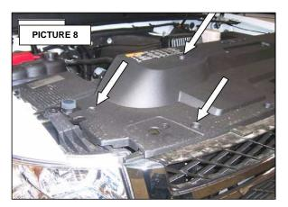
7. Remove the screws securing the top of the grille. Seer picture 9.
