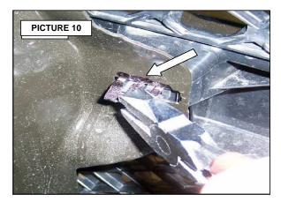
**9.** Remove the bumper bracket bolt from the lop of the driver side frame rail. Align the driver side upper bracket with the hole in the frame and rein stall the bumper bolt. Leave the bolt loose for final adjustment. **See pictures 11 and 12.**
