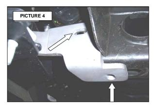
5. Position the tow hook inside the frame, align the bracket and tow hook with the holes in the frame and rein stall the tow hook bolts and nut. Leave the tow hook bolts and nuts loose for final adjustment. See pictures 5 and 6.
